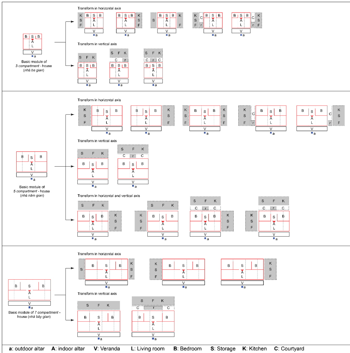
Figure 32 Principle of transformation in the Vietnamese traditional houses in the Mekong Delta.
